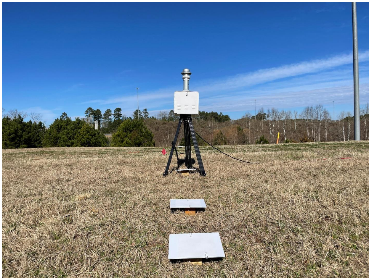
Figure 2. Active air sampler (HI-Q Environmental Products Company, Inc., San Diego, CA, USA) and deposit cards (400 cm 2 , Fisher Pure Cellulose Chromatography Paper, Thermo Fisher Scientific, Inc., Pittsburgh, PA, USA) used to collect triclopyr vapor and particle drift, respectively.
